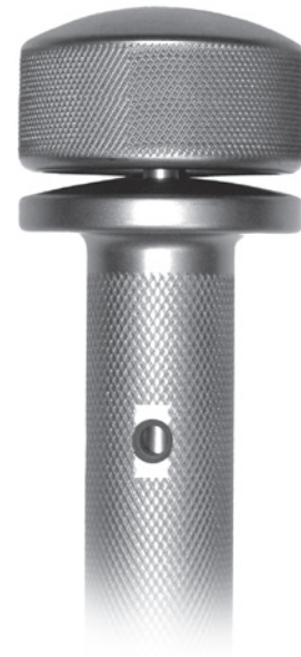
Fig. 14b Strike plate not fully seated against impactor plate
